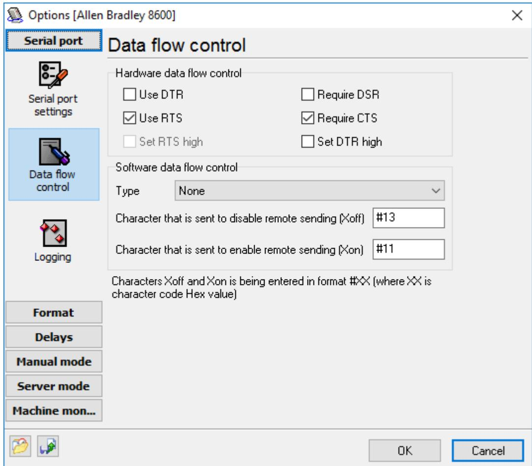
Fig. 3 Handshaking setup.
